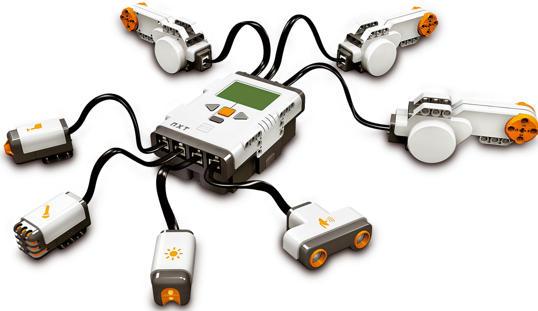
Figure 3.1. Photo of an NXT brick with sensors and motors. 8
