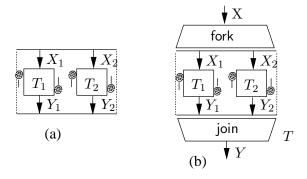
Fig. 10: Interleaved concurrent threads  $T_1$ ,  $T_2$  (a) and composite system T with both join and fork (b).
