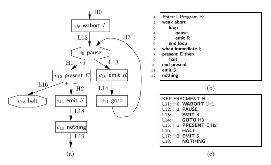
Fig. 8: Sequential Control Flow H (a), Esterel program (b) and KEP Assembler (c).
