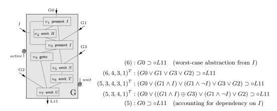
Fig. 7: Component G and some of its WCRT Types with varying precision and conciseness.
