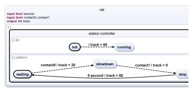
The SCChart describes a simple railway station controller. Initially the track is powered with 60 units to allow any train standing on this platform to begin its journey. (We assume the train stands beyond contact0 and will not trigger it in the beginning.) Subsequently, the platform of this station slows down any train entering the station (indicated by contact0) and stops it when it passes contact1. After 5 seconds it may proceed its journey.
