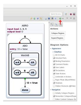
This button will start a new simulation for the model displayed in that diagram view. By default the simulation configuration uses a C code backend for compilation. This requires a GCC available in the system's PATH. If you are using Windows, you need to install some Unix environment (e.g. MinGW or Cygwin). If you want to use a Java backend, you can switch the simulation configuration by clicking on the small black triangle right next to the simulation start button.
