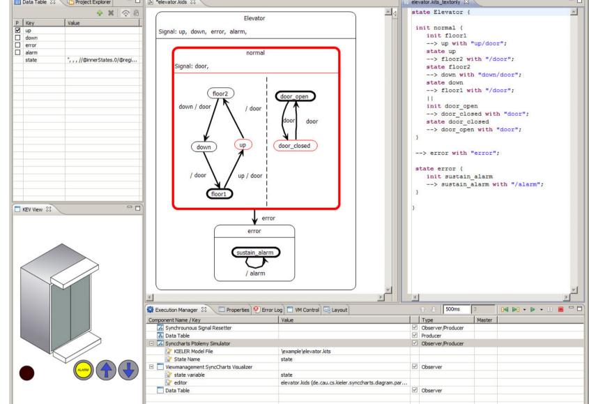
KIELER: Enhancing graphical modeling in Eclipse by integrating into existing frameworks such as EMF, GMF, and TMF [1]
