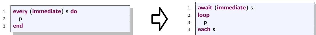
Listing 4.15. The every do statement can be expressed in Esterel by a loop and a preceding await.
