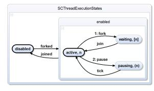
In a trace (see next slide), round/square/no parentheses around n = c.node denote *c.status*, for enabled continuations *c*
