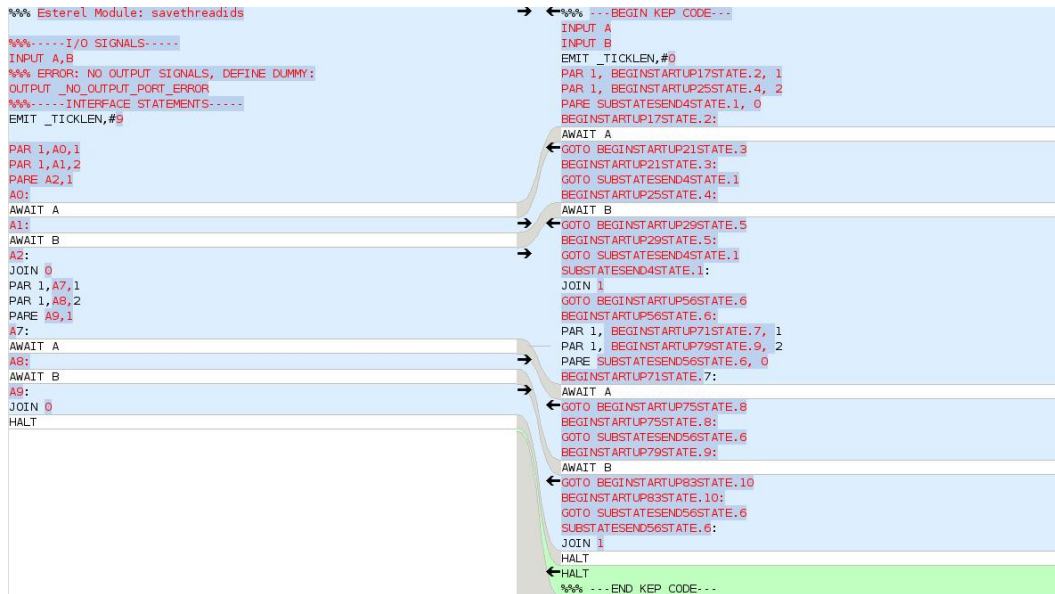
Figure 8.17.: A diff by meld on the KASM code for the thread id saver example. On the left the strl2kasm code, on the right smack! generated code.
