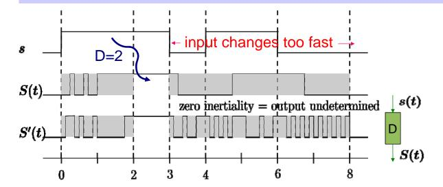
(1) Up-bounded Propagation: If the input remains stable for longer than D time, then the output stabilises to new value.(2) Non-inertial: If input changes, output totally uncontrolled until new value has propagated through.
