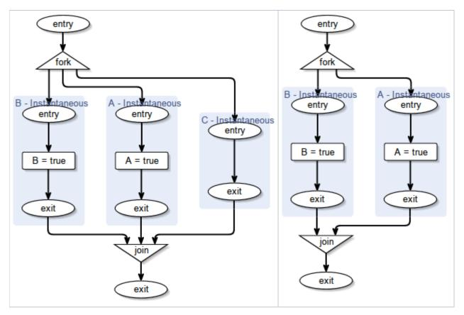
This figure shows that thread C has been removed. If only one thread is left, then the fork and join nodes are removed. If no thread is left, then the parent node from the fork node is connected to the child node of the join node.
