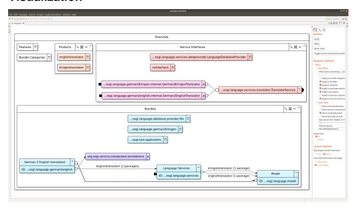
Visualization of parts of a project using the OSGi framework for their architecture
