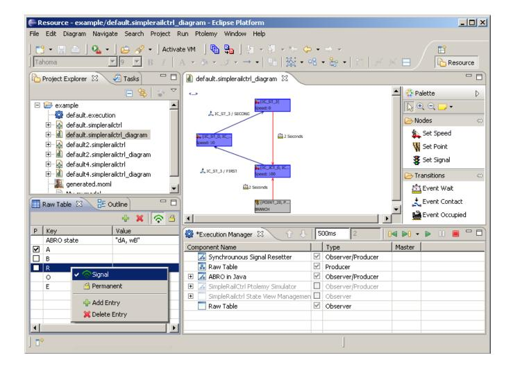
There also exists a demo video that shows the just described behavior. Whenever the execution is being initialized the Ptolemy simulator will transform the currently saved EMF model of the opened diagram into a semantically equivalent but executable ptolemy moml-File.
