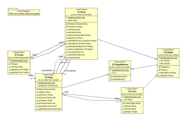
The basic data structure constis of the three classes TNode, TGraph and TEdge, which contain all the necessary properties to model a tree data structure. Therefore a TGraph consits of sets of TEdges and TNodes.
