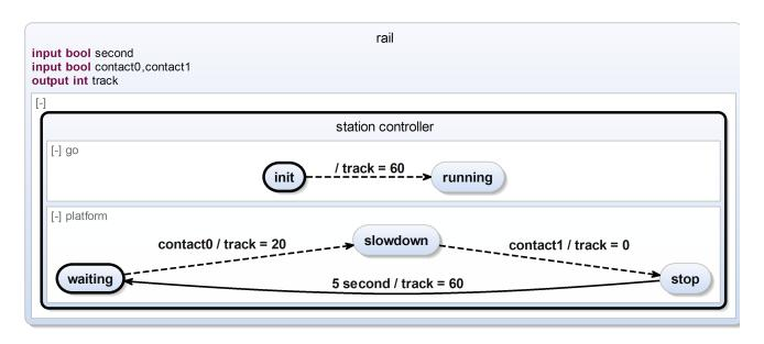
The SCChart describes a simple railway station controller. Initially the track is powered with 60 units to allow any train standing on this platform to begin its journey. (We assume the train stands beyond contact0 and will not trigger it in the beginning.) Subsequently, the platform of this station slows down any train entering the station (indicated by contact0) and stops it when it passes contact1. After 5 seconds it may proceed its journey.
