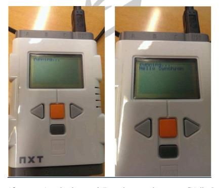
After pressing the (orange) Enter button, the output "Hello Synchron" should appear on the display unit (right photo).
