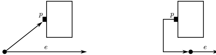
(a) A dummy node placed in the previous layer. The edge e needs to be reconnected and reversed appropriately, and a new edge connects the dummy node with the original target of e .
