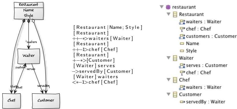
Fig. 1. Different Representations of a Class Model: Diagram, Text and Tree View (created with yUML ( http://yuml.me ) and Eclipse)
