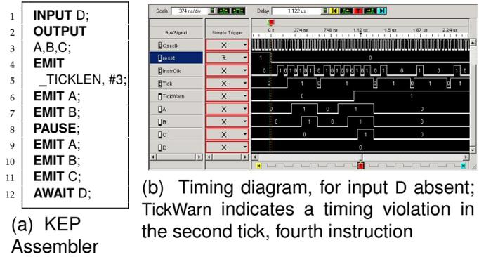
Fig. 6. The Tick Manager detects a timing overrun.
