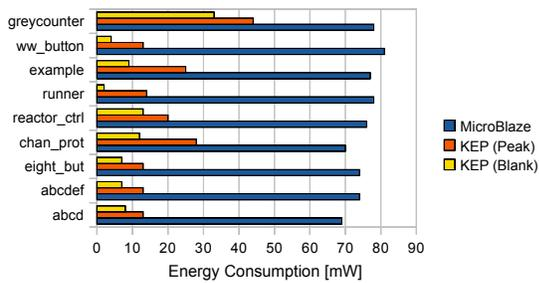
Fig. 10. Energy consumption of KEP and MicroBlaze.
