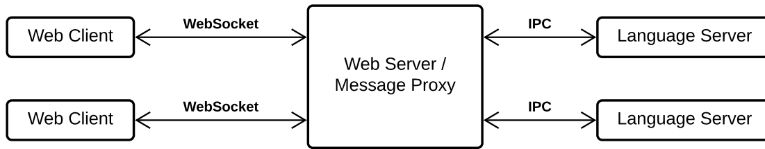
Figure 4.4. Web server that proxies multiple WebSocket connections to language server processes.
