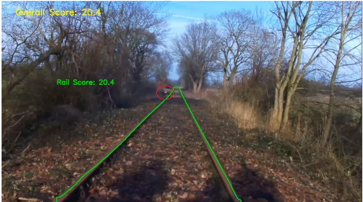
**Figure 6.12.** Field Test: Detection failure case. Poor image quality due to vibrations leads to an overall score of about 20, indicating missed detections under challenging conditions.
