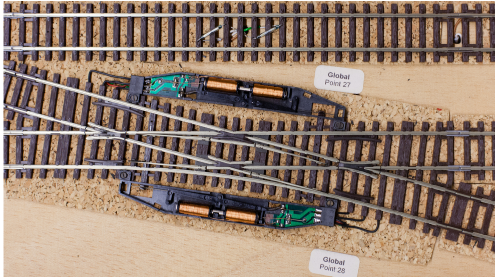
Figure 2.8. Single-slip diamond crossing with opened actuators
