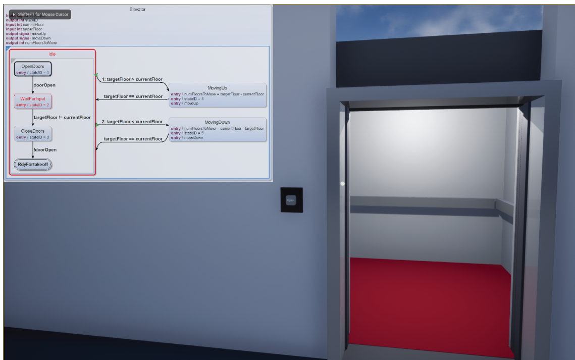
Figure 3.5. The elevator waiting for input
