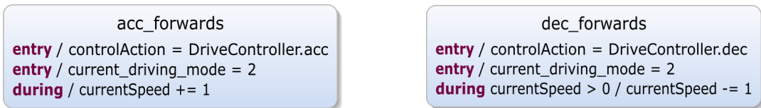
Figure 5.2. States for acceleration and deceleration while driving forwards.
